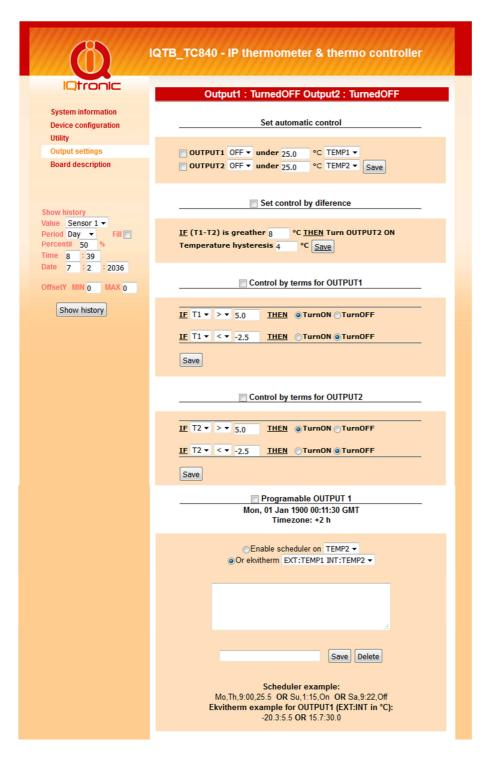
**Set automatic control** - easiest and fastest setup of level monitoring. By using hysteresis of network settings. On each output can be set one sensor value monitoring.
