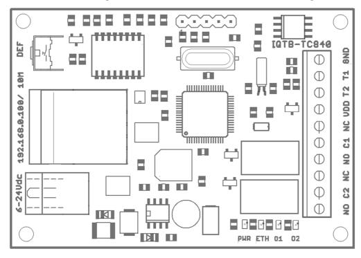
**DEF** This button is for ouputs control – a short press. Or for the factory
