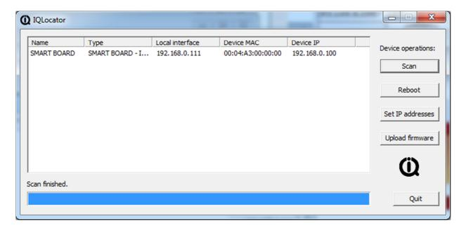
After pressing the button SET IP addresses, we can temporarily change the IP address for configuration directly in the device using a Web browser.
