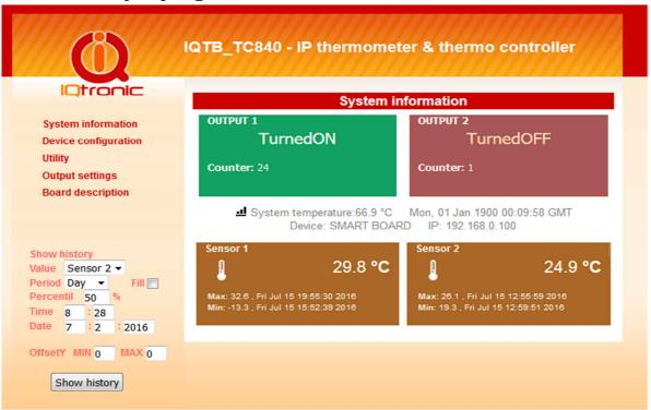
The page will display all data; the current state of the outputs; both of temperature sensors; device temperature; their extreme values; current time obtained from the NTP; status of change counters of outputs. All these values can be read using SNMP protocol version 1.0 or possibly adjust the output relay. It is also possible to set sending TRAP packet in case of exceeding one or more of the conditions.
