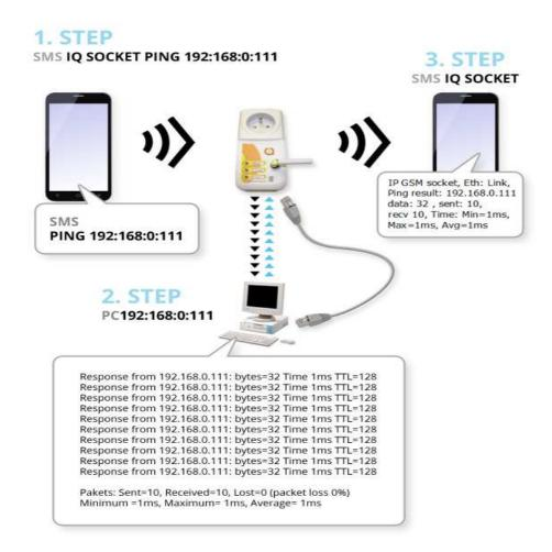
**1. STEP** - send SMS with text PING 192.168.0.111 to phone number to SIM card inserted inside device.
