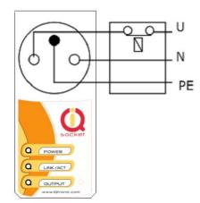
Device uses a single pole relay switch, so it is not performing safe power disconnection of the appliance plugged into socket, only functional switching is performed.
