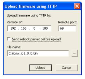
After browsing the target file containing new firmware and clicking to "Upload" button, a progress bar will be displayed. Green Link LED indicator will blink during upload process.
