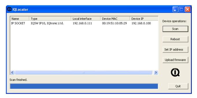
In order to change device IP address, select particular device by clicking to the row and then click to button "SET IP addresses" button:
