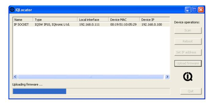
When upload is finished, a confirmation message "Successful" will appear and now it is necessary to wait about 30seconds till internal firmware rewrite procedure finishes, during which the Power LED (red) will blinking fast. Then an automatic reboot of device will be performed and device is ready for use now.
