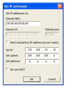
Once you enter new IP address and click to "Set" button, a confirmation message "IP address was successfully set" will be displayed and new SCAN process will be performed to locate your device with new IP address. This IP address setting is temporary, valid until next device start. To make change IP permanent, it is necessary to use WEB management (see chapter Chyba! Nenalezen zdroj odkazů.) to save changes permanently.
