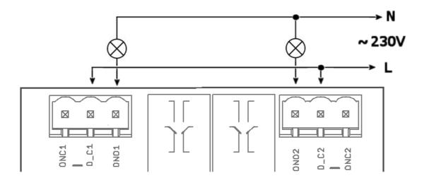
Your device has two independent non-potential NO/NC outputs with the maximum load of **16A** (resistive) for 230VAC voltage, which are the output contacts for the relays.
