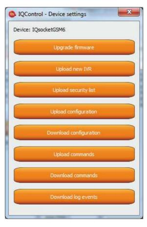
Upgrading the internal firmware.
