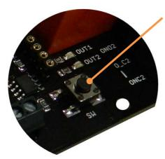
An integrated micro push button is located at the device, can be accessible directly by finger.It named with the text "SW".
