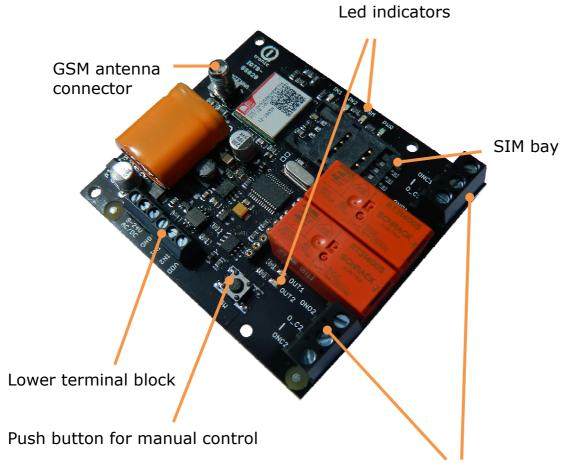
Terminal block with 230VAC input and power relay ouputs
