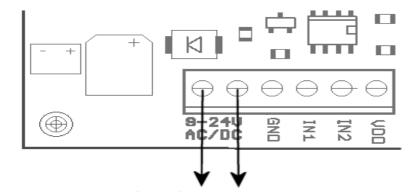
Connect this pins to power supply. It can be powered by AC or DC voltage.
