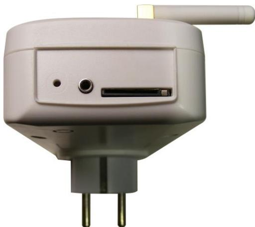
An integrated micro push button is located in the device, can be accessible through a round hole of 2 mm at the most outer side of your socket.
