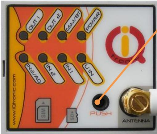
An integrated micro push button is located in the device, can be accessible through a round hole of 3 mm named with the text "PUSH".
