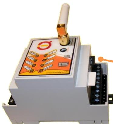
Your IQTD-GS400 offers an option to save all log events at the given time in detail into the SD card inserted into SD card bay. The maximum size is 4GB and the card must be formatted. The **FULL license** is required.
