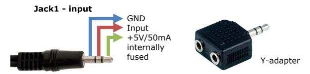
There is provided +5V/50mA power supply line for powering external sensors.
