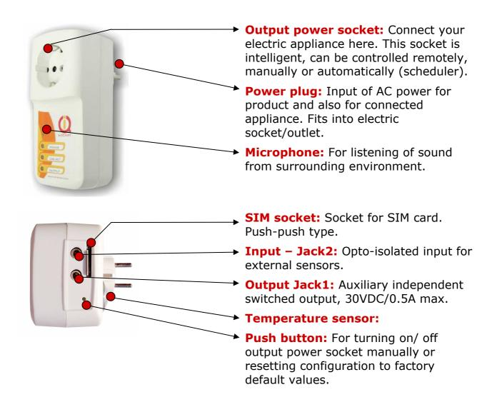
Besides controlling of the power, IQsocket IQSW-GSM is equipped with a choice of useful functions, including:
