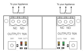
(switch positions drawn on the picture are in Turned Off state)
